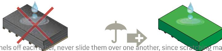
Always lift panels off each other, never slide them over one another, since scratching may occur. To carry the panels, stand them on their back edge and lift with a minimum of two people (one person at each end) protecting the face from scratching or damage. Always lean panel towards back edge to avoid damaging visible front edge. Using soft bearers can help to rest the panel edge on.
